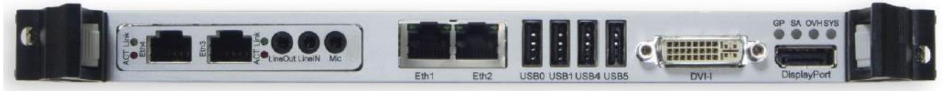
Figure B-7 – View of the CPC505 front panel with the MIC1901 module installed
